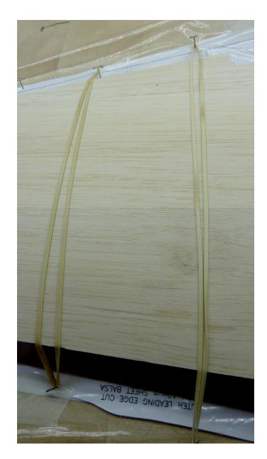
This detail shows two pairs of pins and rubber bands in place.
